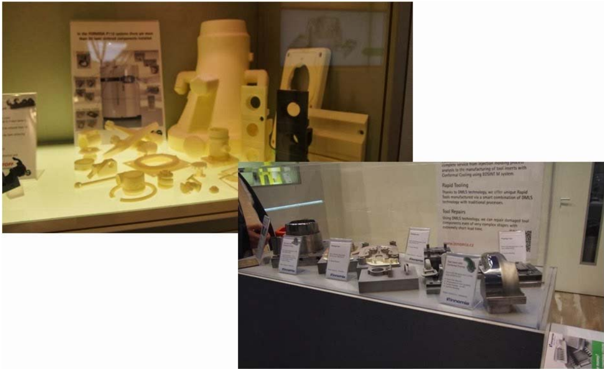
Fig.6 Samples at EOS's booth Left: Laser sintered plastics samples Right: Laser sintered metal samples (mold parts)
