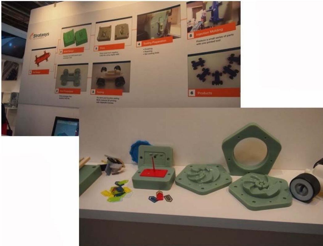
Fig.2 Explanation panels, resin molds made from inkjet process and injection molded samples at Stratasys's booth
