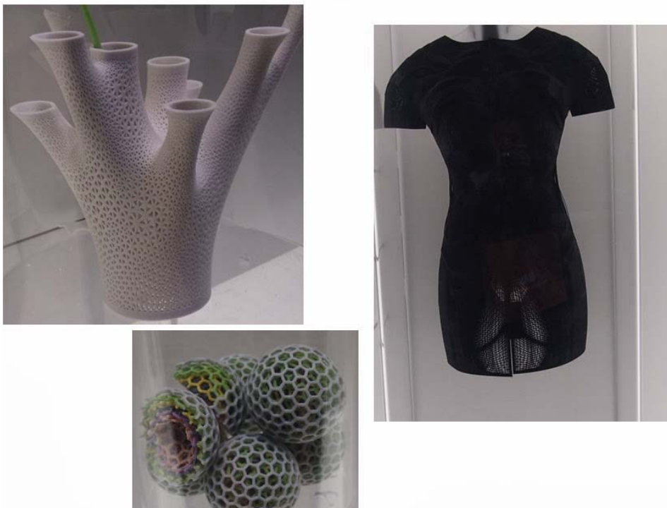
Fig.4 Samples at Bayer's booth (2) Samples made of thermoplastic urethane power
